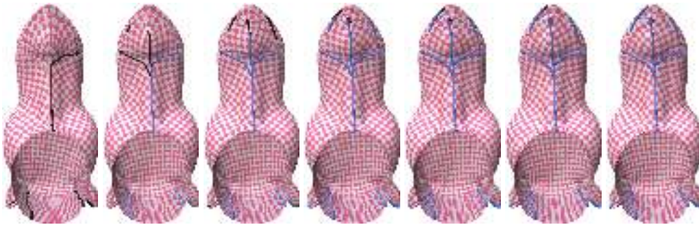
FIGURE 5.16: Results after multiple runs of our algorithm. This enables us to capture some natural cuts that our algorithm may have missed. After a few runs cuts our method converges, and the cuts stop expanding.
