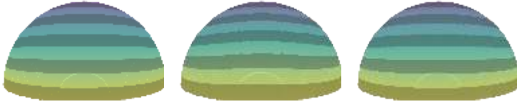
FIGURE 2.23: Laplace problem on a half sphere, discretized with grid-step h = 0.01 (95445 surfels). We start from a linear function: left picture is both the integrated function and the expected result, as this is a spherical harmonic. Middle is the result obtain with a non corrected Laplacian: there is small visible distortion, as well as global distortion (isolines are not parallel to the border of the half sphere). On the right, results are obtained with a corrected operator: while there is still some small distortion, isolines are parallel to the border.
