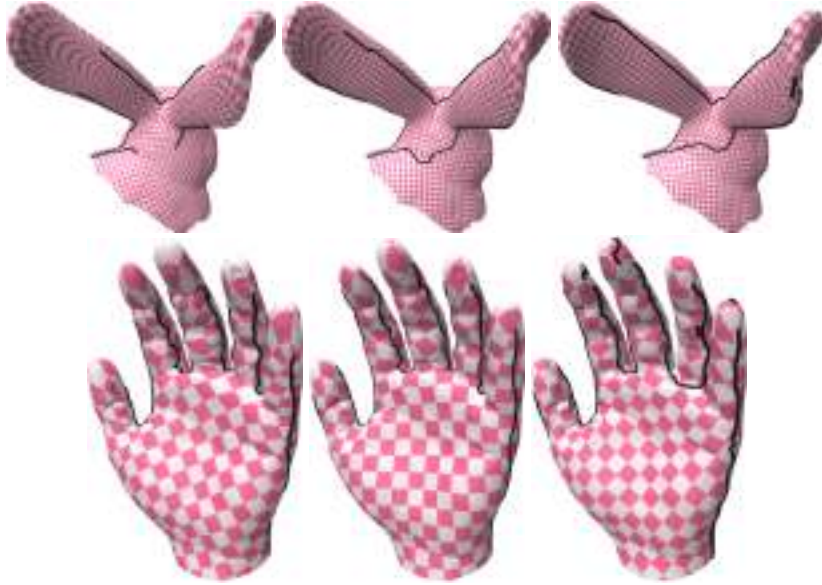
FIGURE 5.15: Results on the bunnyhead and hand meshes for \lambda = \{3, 1, 0.1\} (reps. from left to right). Lower \lambda parameter implies longer cuts.
