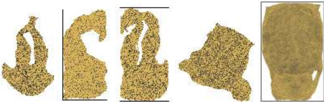
FIGURE 5.18: Resulting parameterizations without bounding box constraints (a, d) and with bounding box (b, c, e) on the bunnyhead and david mesh. The first example with bunnyhead (b) does not have border injectivity restrictions, enabling the many overlaps which are not present on the second example (c) (which has border injectivity restrictions). On the david mesh, an overlap free parameterization was obtained (e) without using our border injectivity restrictions, giving the same result with our without them.
