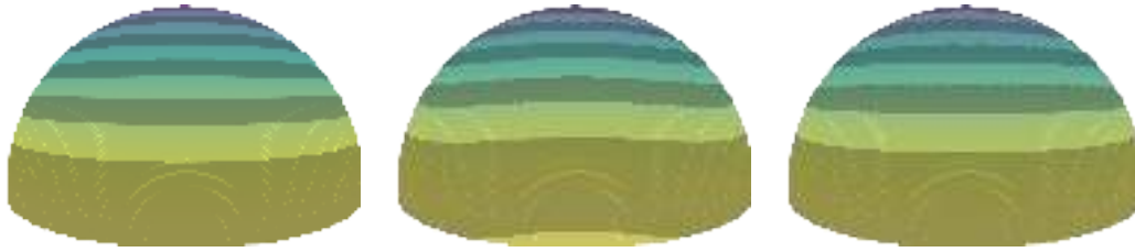
FIGURE 2.24: Laplace problem on a half sphere, discretized with grid-step h = 0.01 (95445 surfels). We use a higher spherical harmonic than figure 2.23. Again, left is both the integrated function and the expected result, middle is obtained without correction and right is with. The distortion is visible in both case, however the shape of the corrected function is visibly better than the non corrected one.
