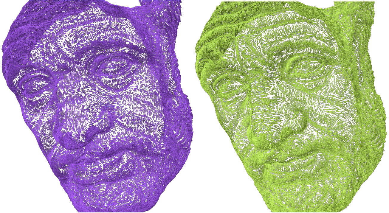
Figure 1: First and second principal directions on scanned data (from https://threedscans.com ), using CNC-Avg-Hexagram with K = 50 , objects is composed of 499500 points.
