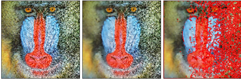
Fig. 3. In this figure we have added a spatially-variant noise to the Mandrill image. In this case it is not possible to find an optimal (\alpha, \lambda) pair that denoises and segments the image appropriately with our current model.
