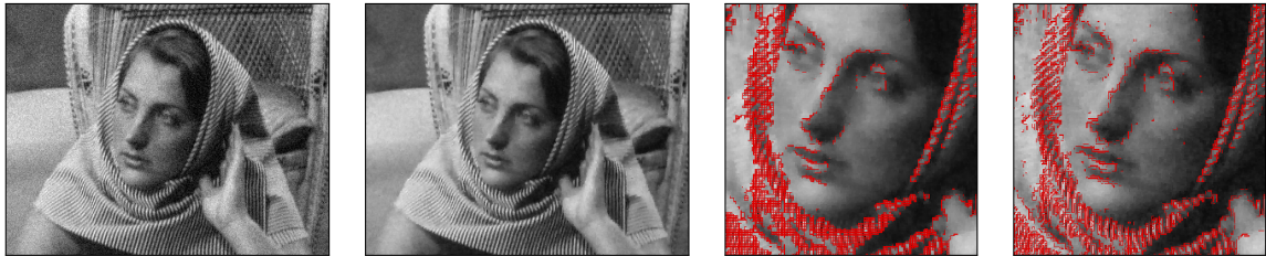
Figure 5: Input corrupted with Gaussian noise \sigma = 0.1 (first column), restoration (second column), contours with AT_\epsilon^{0,1} , \lambda = 0.0054088 and \alpha = 1.0 ; contours with AT_\epsilon^{2,0} , \lambda = 0.0064905 and \alpha = 0.69 . For both, \epsilon \in [1, 0.25]
