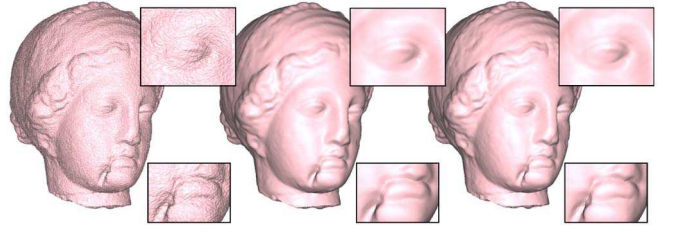
Fig. 4. Left: an noisy input model. The local, iterative scheme, with both spatial weighting term W_c and signal weighting term W_s (Right) gives better denoising results than with only signal weighting term W_s (Middle).
